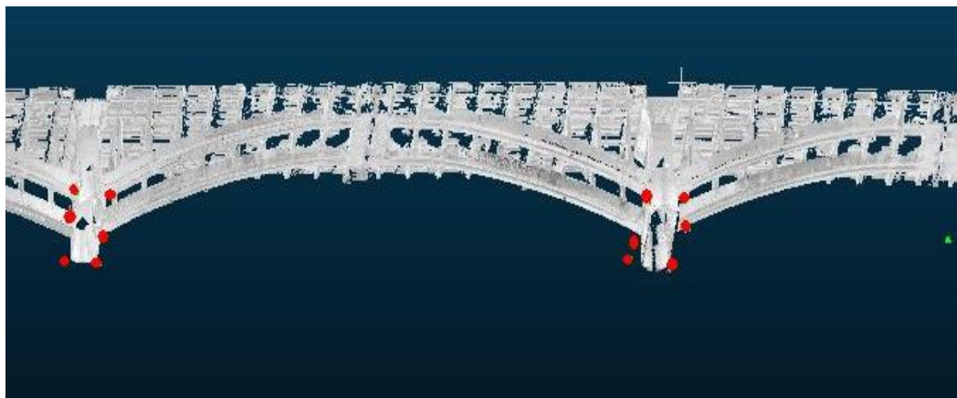
Figure 1 — Sample cloud of bridge transition points (approx. 420 million points)
